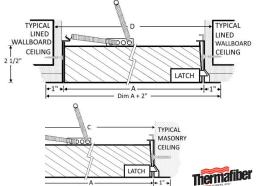
WALL INSTALLATION 1-1/2 HOUR UL"B" LABEL IN A 2 HOUR FIRE BARRIER Use "C" Dimension for Installation Without Wallboard Liner Add 1-5/8" to "A" for 5/8" Wallboard Liner of Opening on 4 Sides
