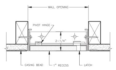
Our recessed drywall door gives the option of installing a matching piece of drywall into the door panel thus keeping the continuity of the visual area.
